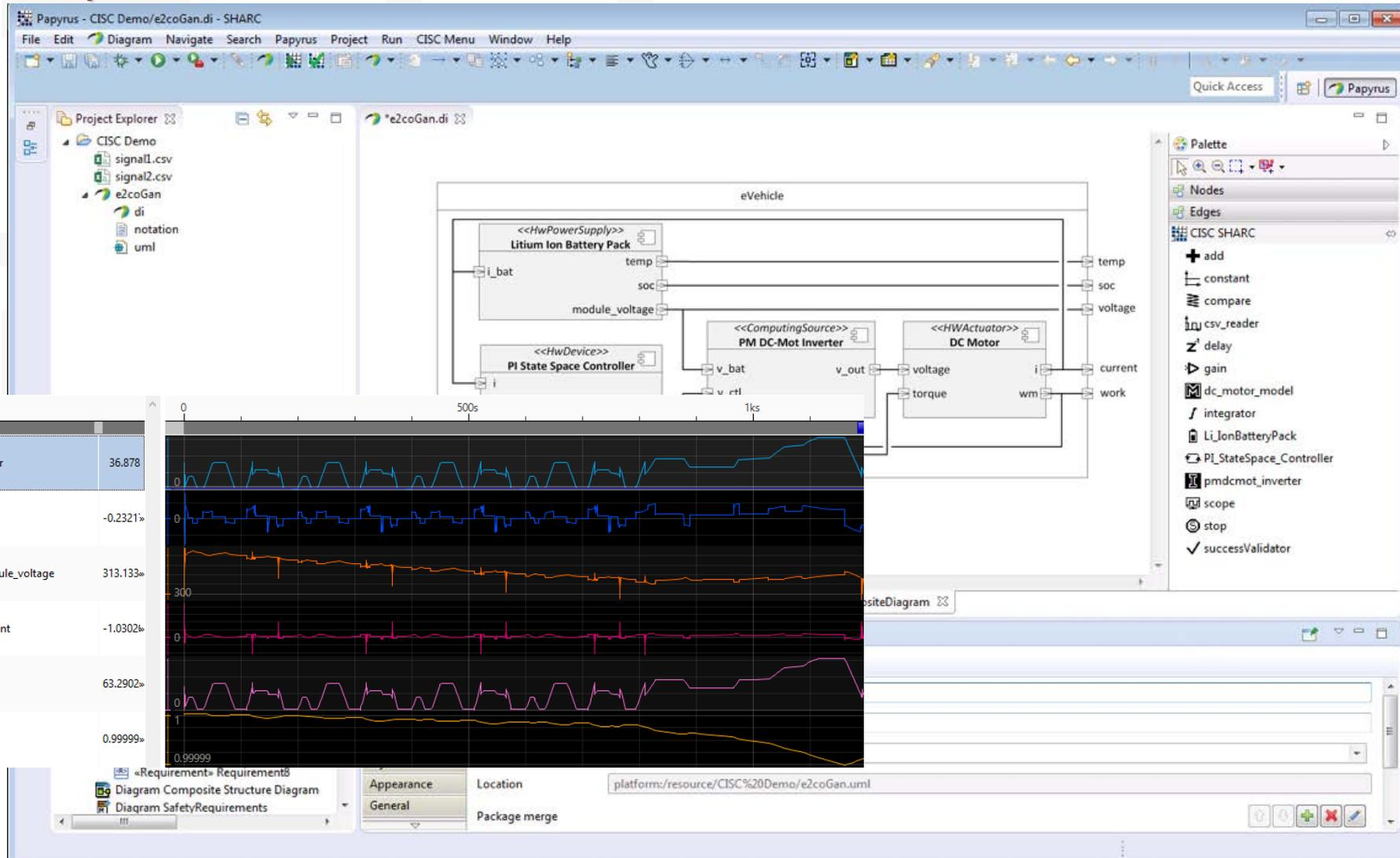
The screenshot displays the Papyrus IDE interface for a CISC SHARC project. The main workspace shows a system architecture diagram for an 'eVehicle' system. The diagram includes several components:
