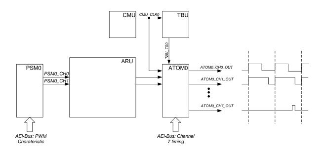
**Figure 1.1:** Flexible PWM generation with the ATOM submodule.
